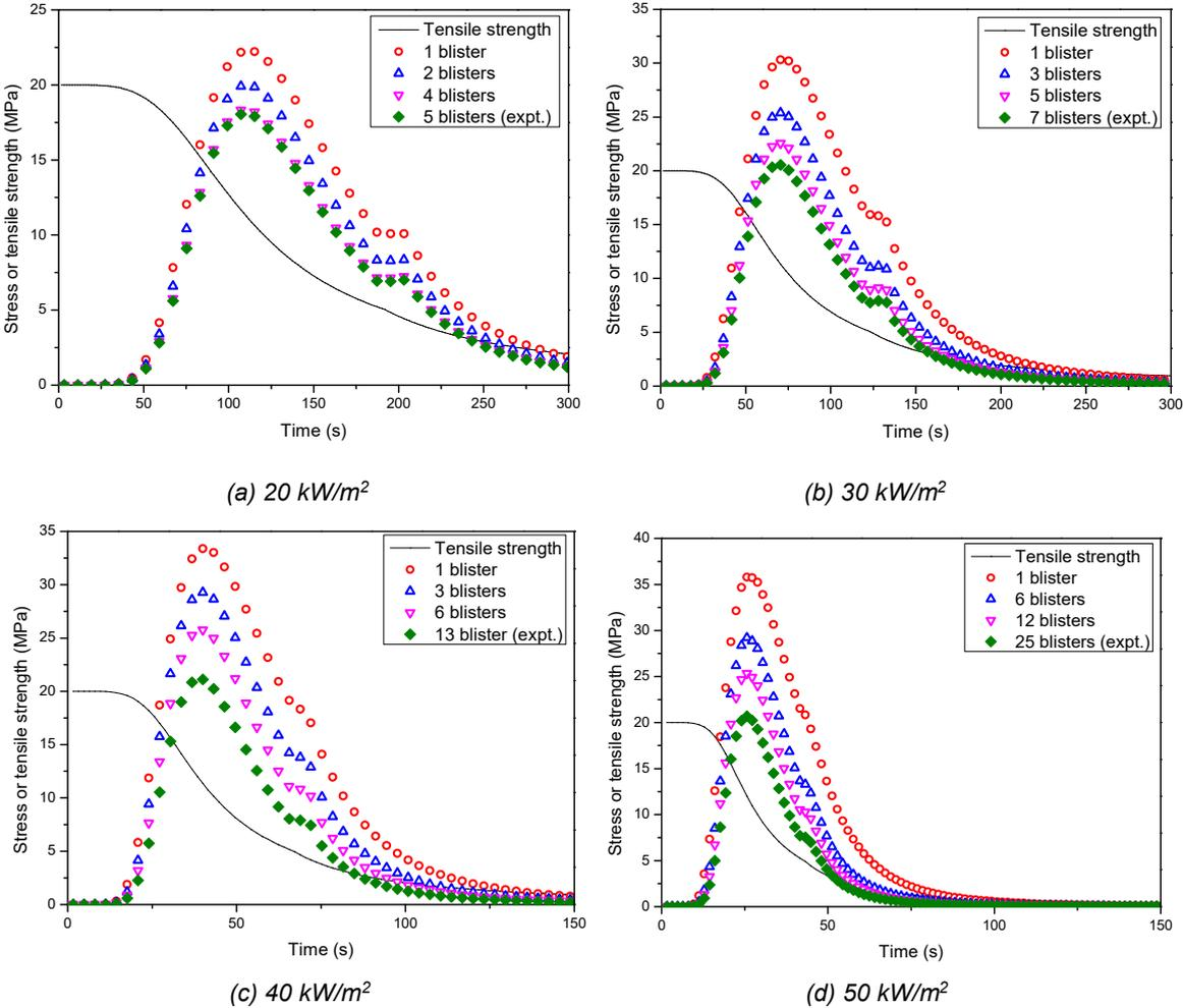
Figure 3: Surface stress and tensile strength
