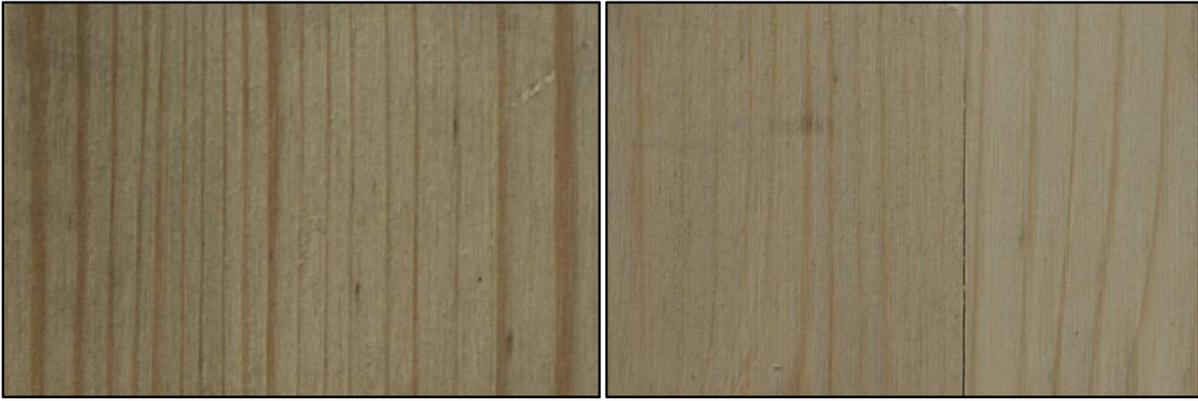
Figure 3: Grain direction variation in CLT samples with low (left) and high (right) variability
