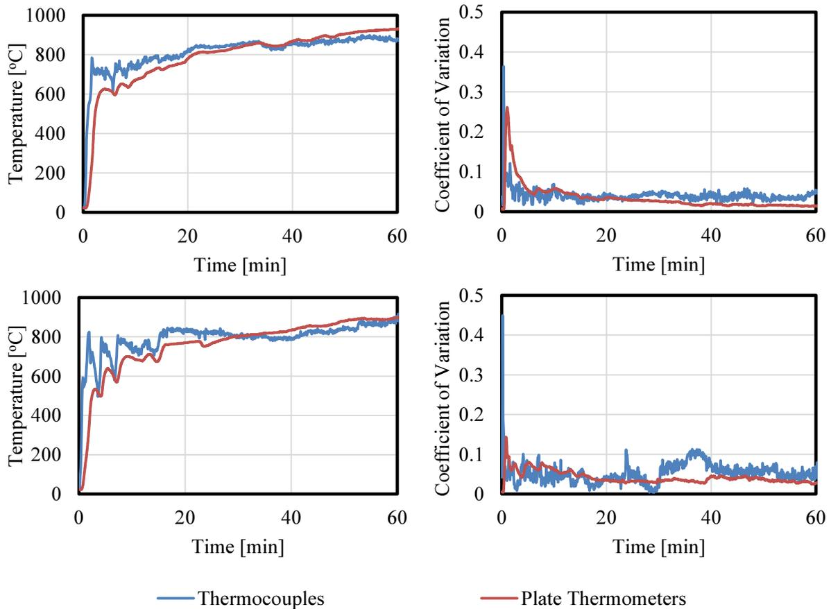
Figure 1: Temperature data for two furnace tests as measured by thermocouples and plate thermometers, showing coefficients of variation for each
