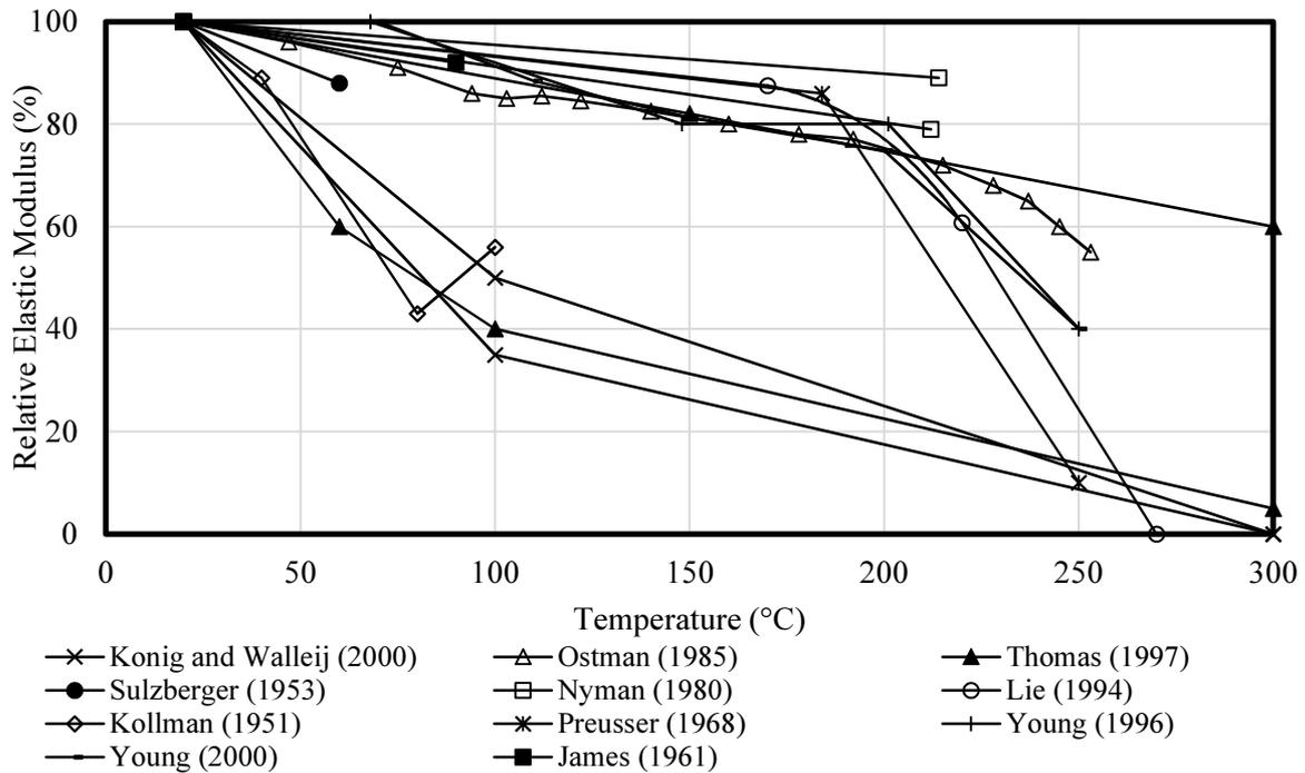
Figure 2: Temperature-dependent elastic moduli from different researchers
