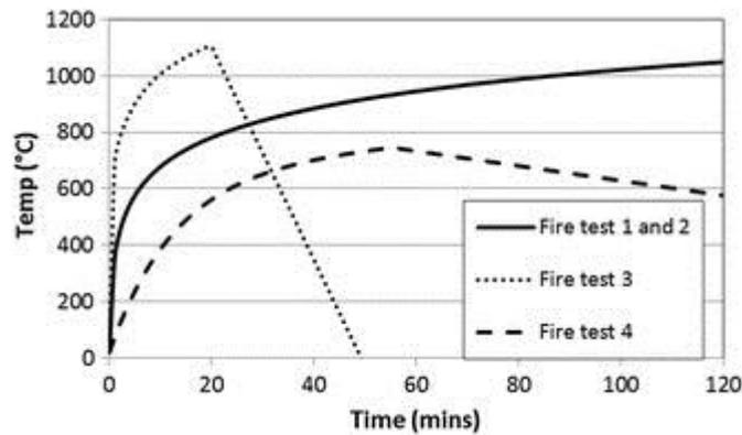
Figure 3. Time-temperature fire curves of tests presented in (Lange et al. 2015).
