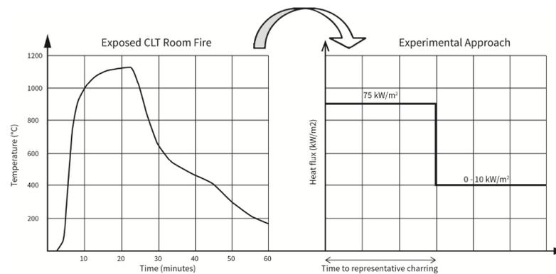
Figure 4. Temperature load of fire tests converted to heat flux to the surface loads (Roy 2015).
