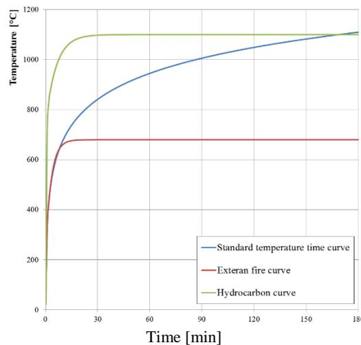
Figure 1. Different nominal fire curves specified in EN 1363-1.
