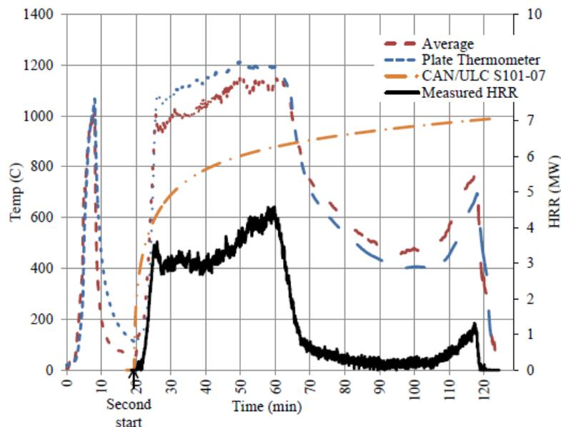
Figure 2. Time-temperature fire curves and HRR of tests presented in (McGregor 2013).
