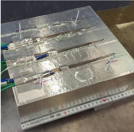
Figure 3: Aluminium tape around the specimen
