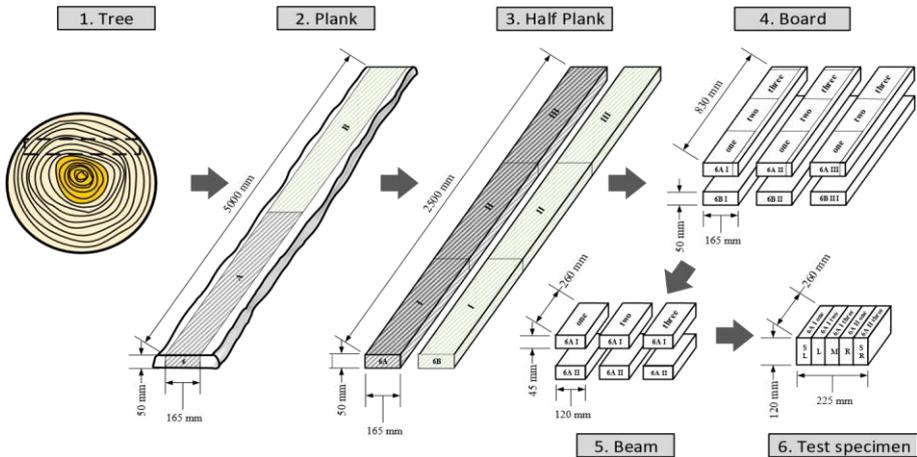
Figure 1: Scheme of the specimen production.
