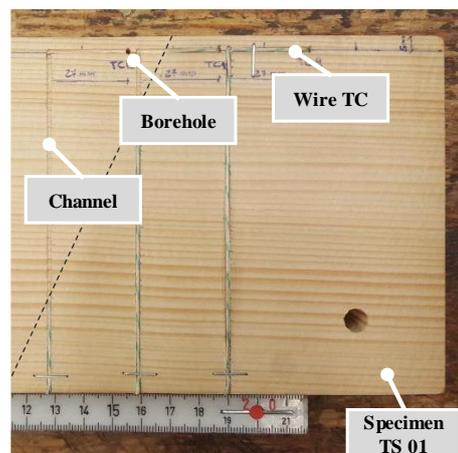
Figure 4: Installation of the inlaid wire thermocouples (TCs) in the specimen TS01.
