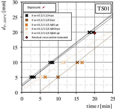
Figure 12: Char-line depth-time relationship of the specimen TS01.
