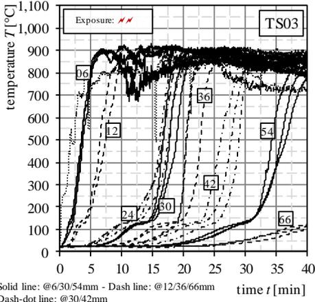
Figure 10: Temperature time relationship in the specimen TS03; legend see Figure 11.
