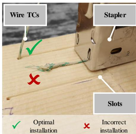
Figure 3: Installation of the wire thermocouples (TCs) in specimen TS03.
