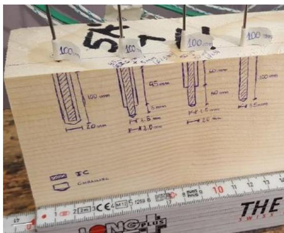
Figure 6: Installation of insulated tube thermocouples in boreholes.
