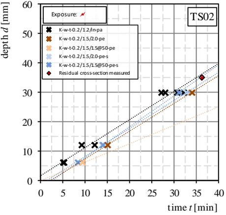
Figure 13: Char-line depth-time relationship of the specimen TS02.
