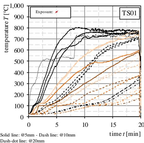
*Figure 8: Temperature time relationship in the specimen TS01; legend see Figure 11.*
