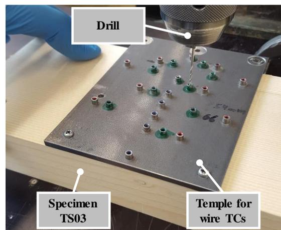
Figure 7: Drilling of boreholes to install the wire thermocouples (TCs).
