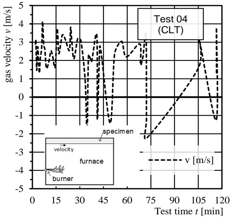
Figure 11: Determined gas velocities in the model scale furnace of VKF, Switzerland (formerly EMPA).
