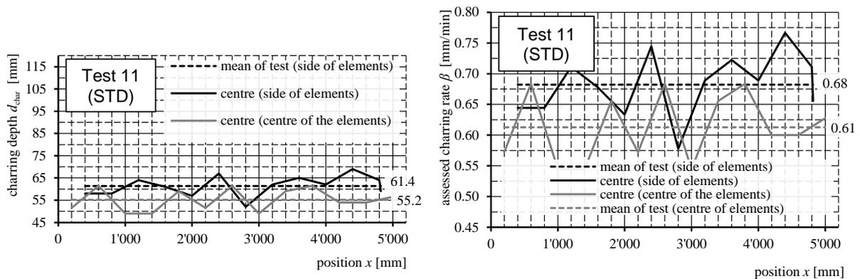
Figure 9: Assessment of the charring depth (left) and rate (right) using both measurement techniques.
