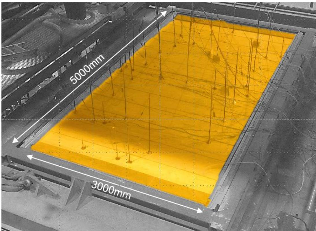
*Figure 2: Test specimen installed on the horizontal full scale furnace at the fire lab of Rise.*
