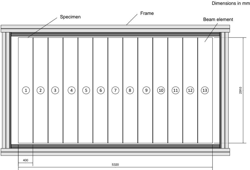
Figure 1: Test specimen assembled out of beam elements and the metal frame with fitting layers.
