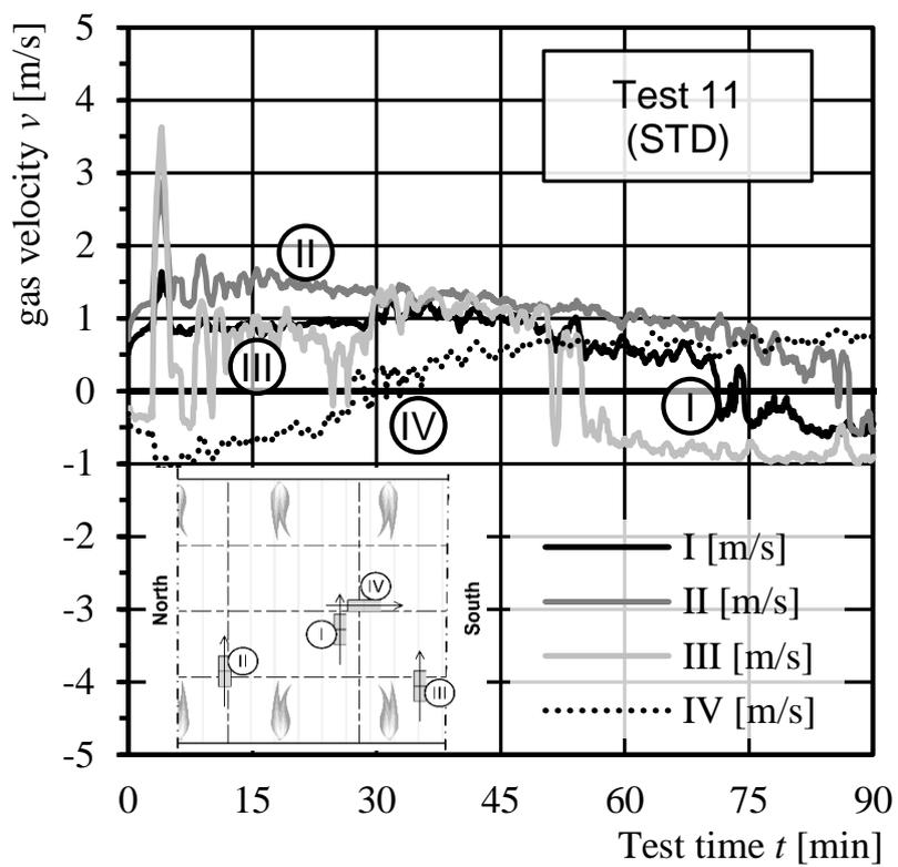
*Figure 12: Determined gas velocities in the full scale furnace of Rise, Sweden (formerly SP).*
