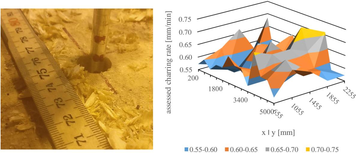
Figure 5: Measurement device (left). Assessed charring rates using the special made meter (right).
