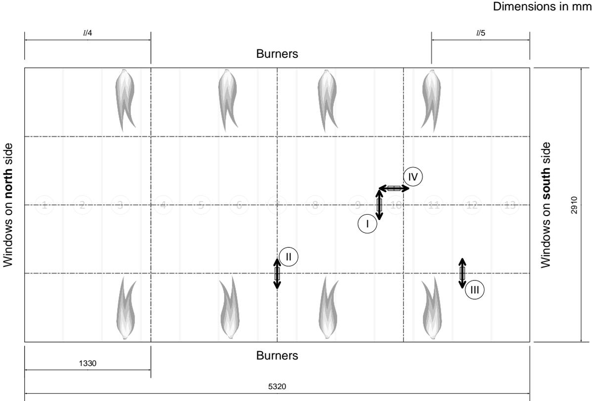
Figure 3: Pitot tubes I to IV and burner location in the specimen.
