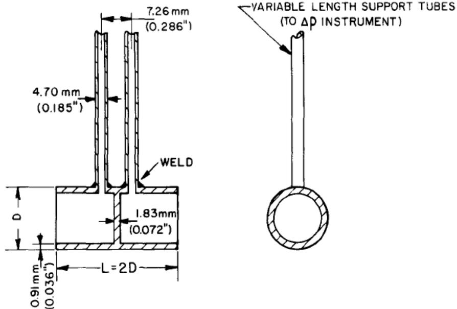
Figure 10: Pitot tube type used in the furnace test (image by McCaffrey et al., 1976).
