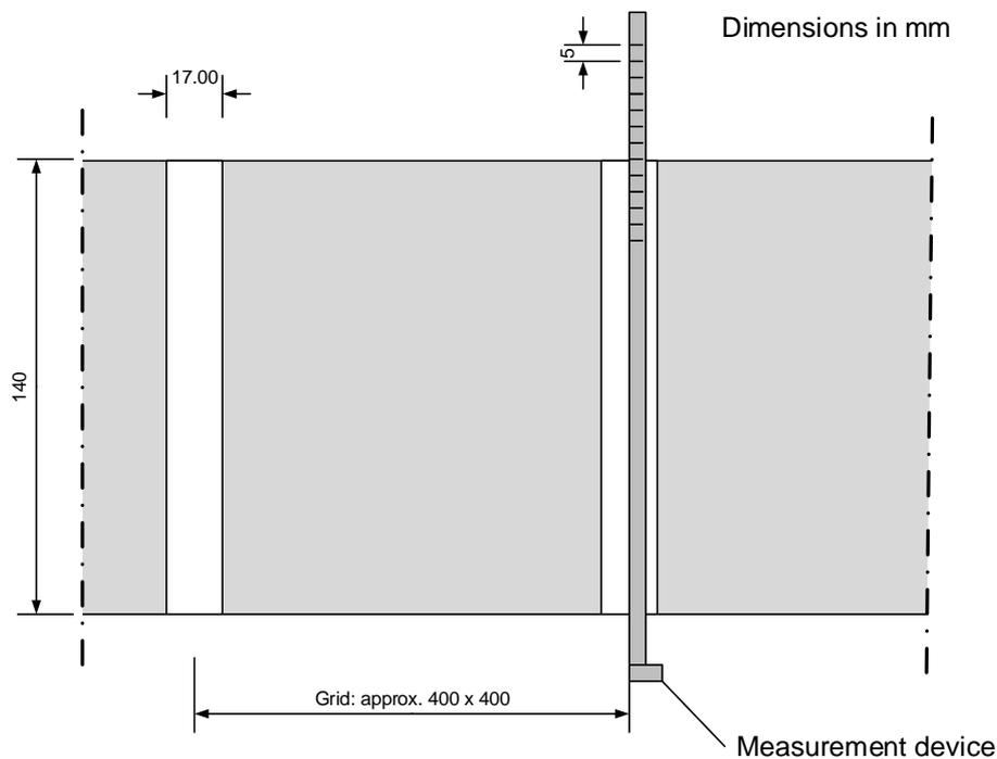
Figure 4: Measurement of the residual cross section. Vertical channels were drilled along the centre line.
