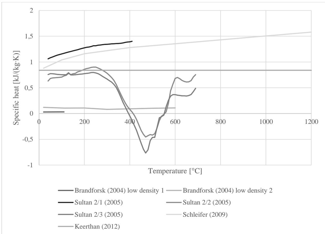
Figure 11: Specific heat of stone wool insulation according to literature
