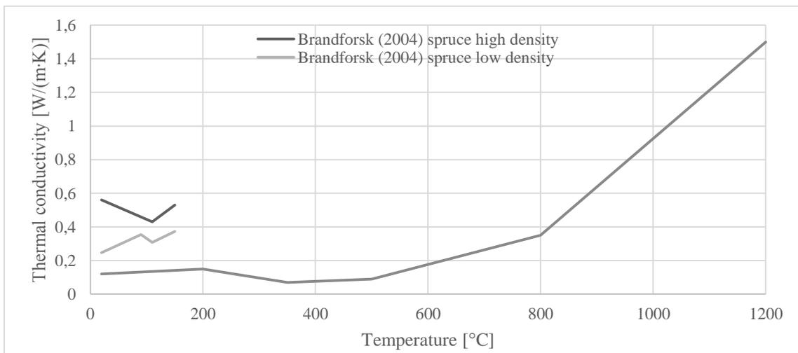
Figure 13: Thermal conductivity of timber according to literature
