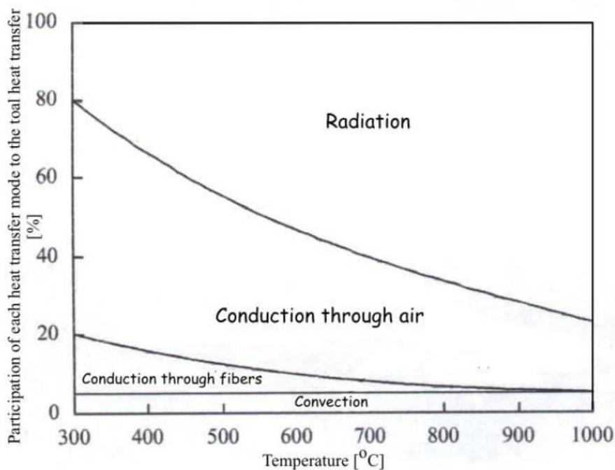
Figure 20: Heat transfer mechanisms in fibrous insulation materials according to [11]
