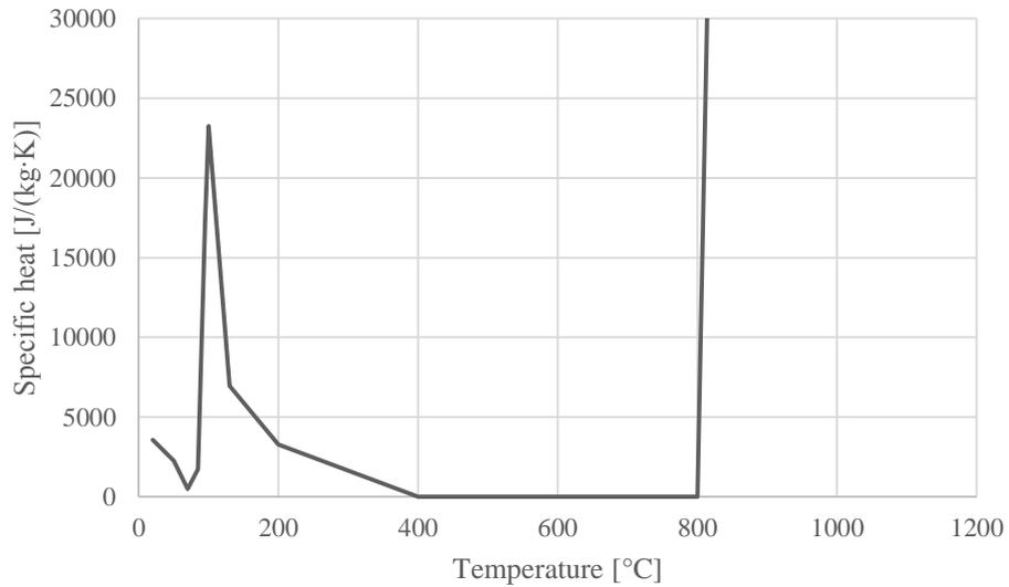
Figure 22: Specific heat of a loose fill cellulose fibre insulation
