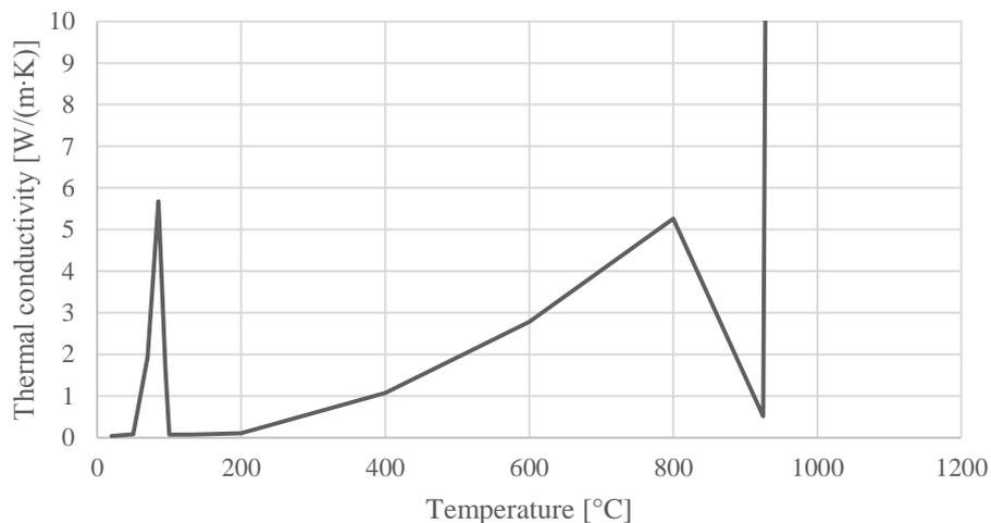
Figure 21: Thermal conductivity of a loose fill cellulose fibre insulation
