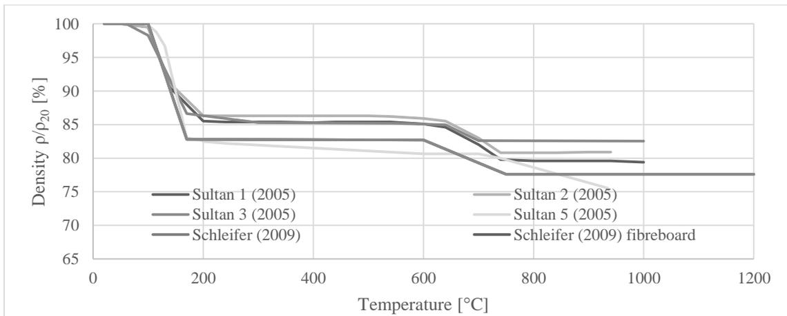
Figure 8: Density ratio ( $\rho_T/\rho_{20}$ ) of gypsum plasterboards and gypsum fibreboards according to literature
