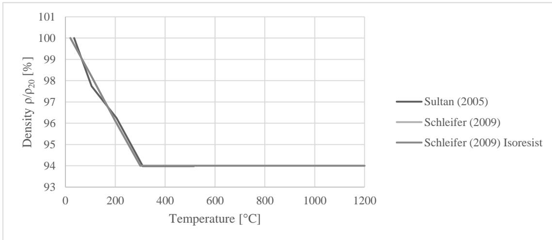
Figure 4: Change in density ratio ( $\rho_T/\rho_{20}$ ) of glass wool insulation from literature
