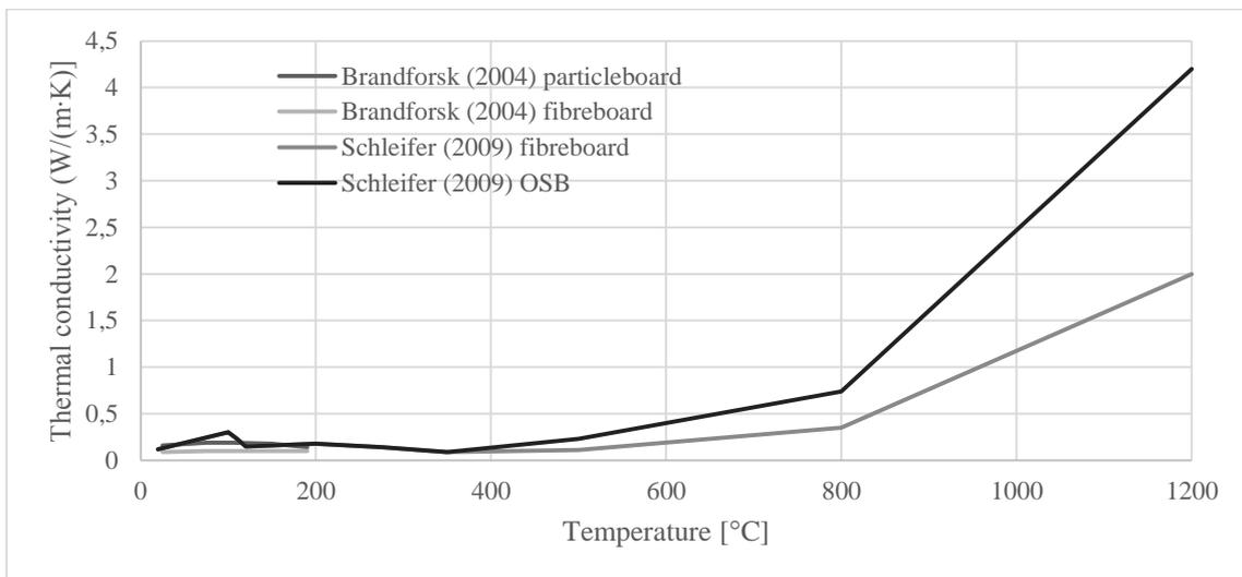
Figure 16: Thermal conductivity of wood-based boards according to literature
