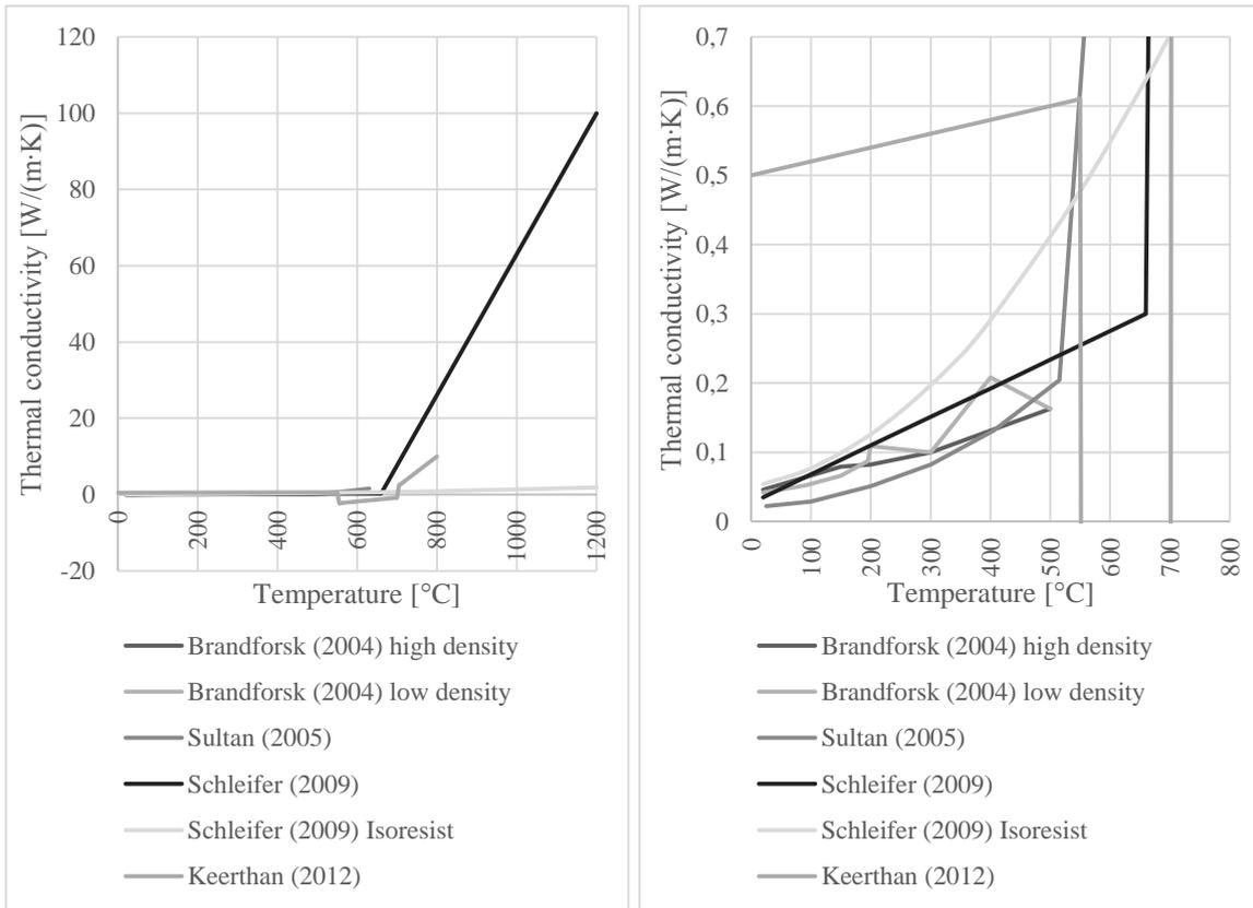
Figure 2: Thermal conductivities of glass wool insulation from literature (full graph on the left, fragment on right)
