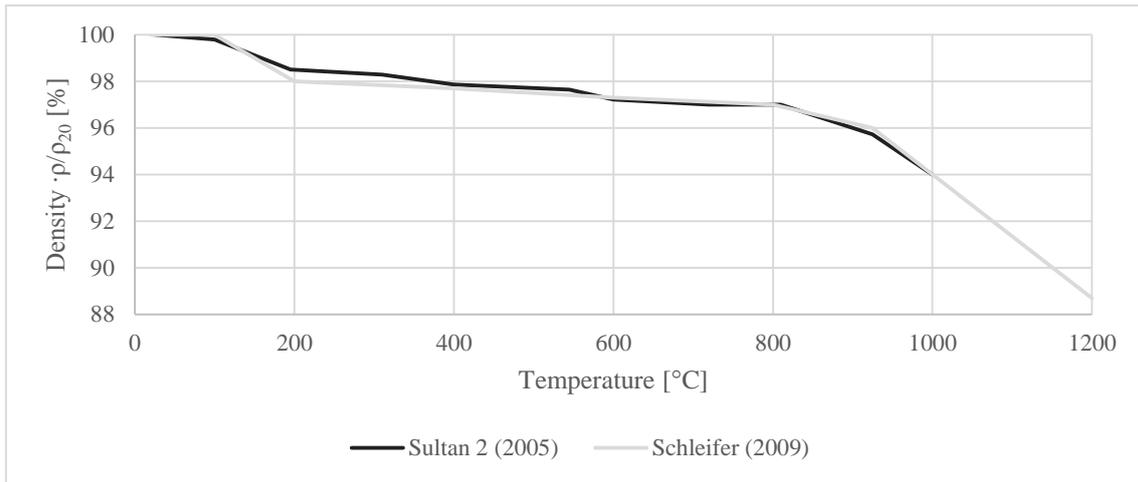
Figure 12: Density ratio ( $\rho_T/\rho_{20}$ ) of stone wool insulation according to literature
