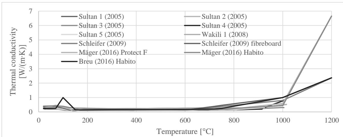
Figure 5: Thermal conductivity of gypsum plasterboards and gypsum fibreboards from literature
