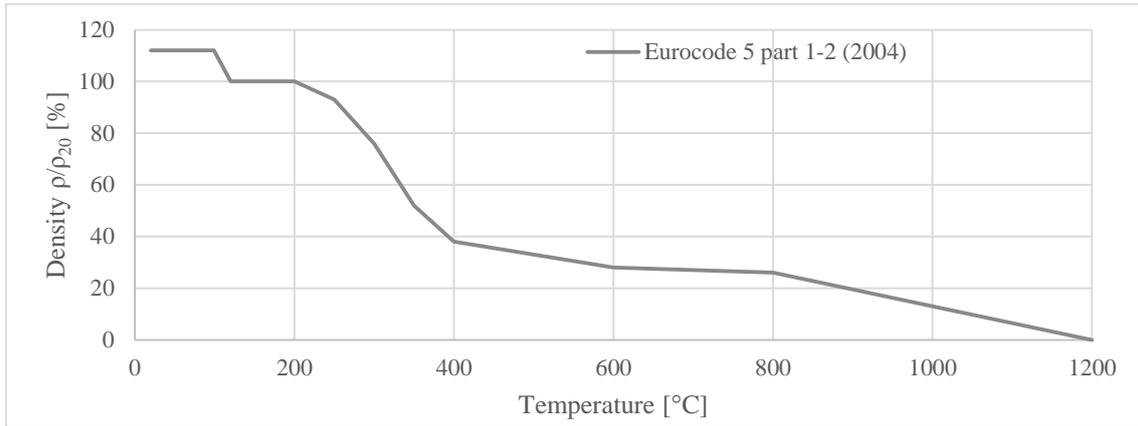
Figure 15: Density ratio ( $\rho_T/\rho_{20}$ ) of timber according to literature
