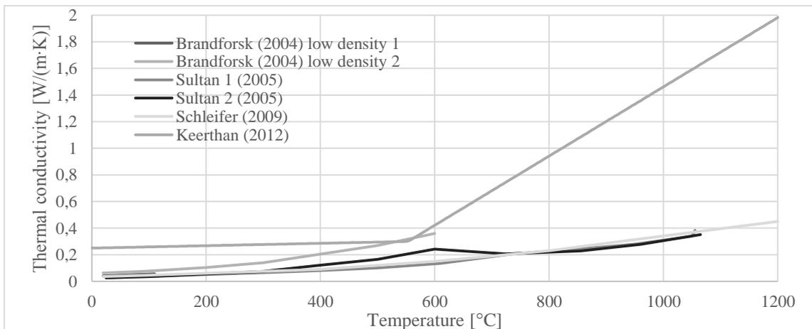
Figure 9: Thermal conductivity of stone wool insulation according to literature
