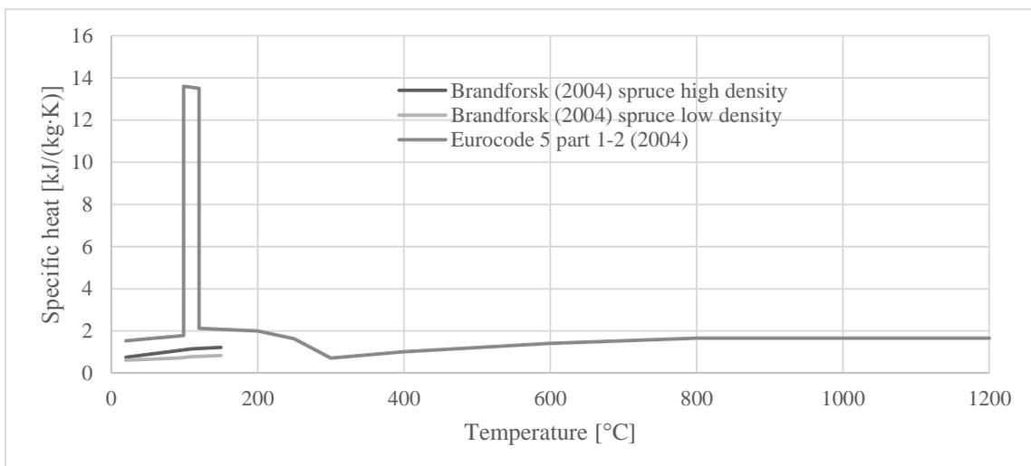
Figure 14: Specific heat of timber according to literature
