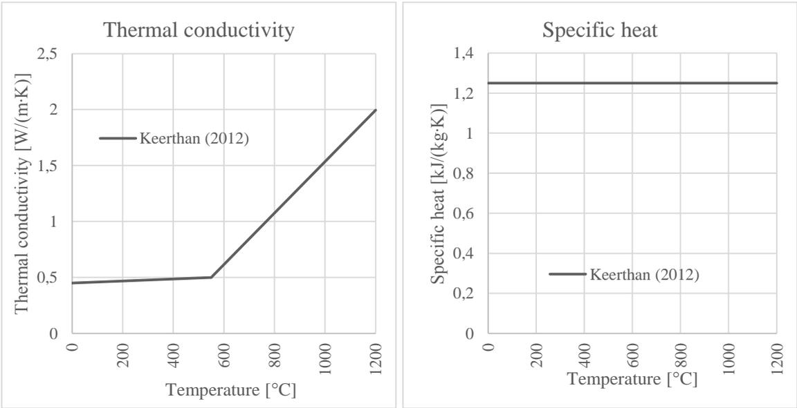
Figure 1: Thermal properties of cellulose fiber insulation from literature
