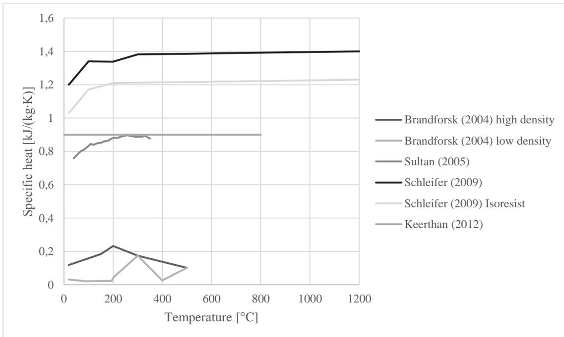
Figure 3: Specific heat values of glass wool insulation from literature
