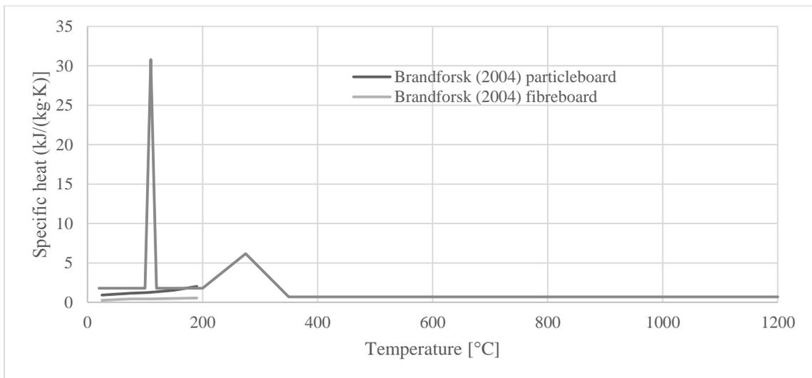
Figure 18: Specific heat of wood-based boards according to literature
