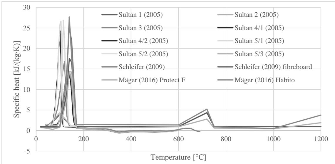
Figure 7: Specific heat of gypsum plasterboards and gypsum fibreboards according to literature
