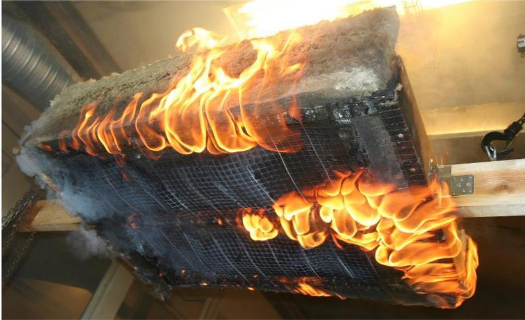
Fire test of unprotected loose fill cellulose fibre insulation fixed with chicken net and steel bars
