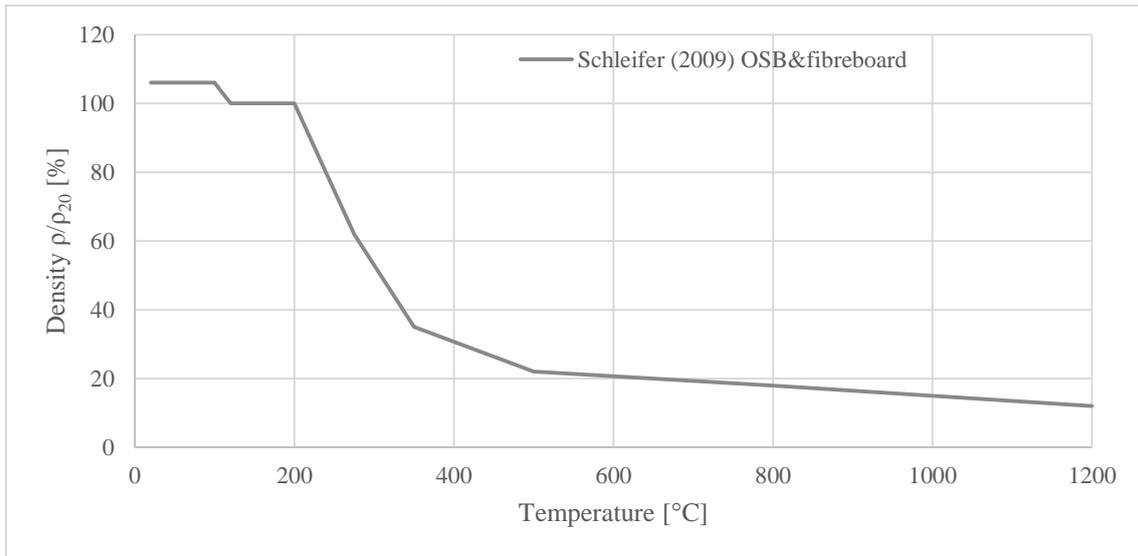
Figure 19: Density ratio ( $\rho/\rho_{20}$ ) of wood-based boards according to literature
